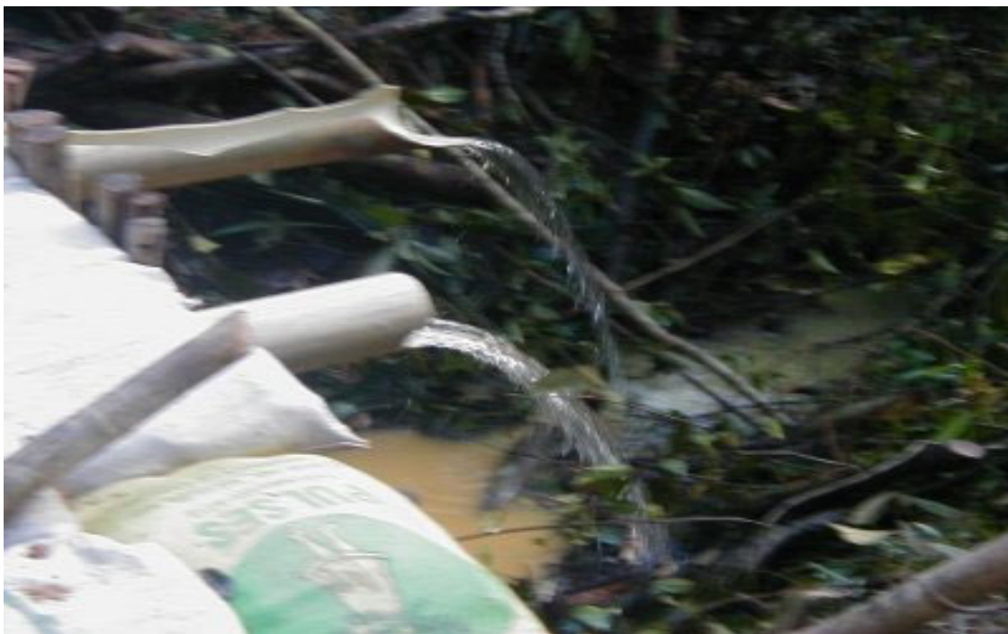
Figure 2: An example of ‘good’ mining practice. Water discharged from the Tailings Pond indicate very low level of sediments. (Pictures with compliments of GGMC)
