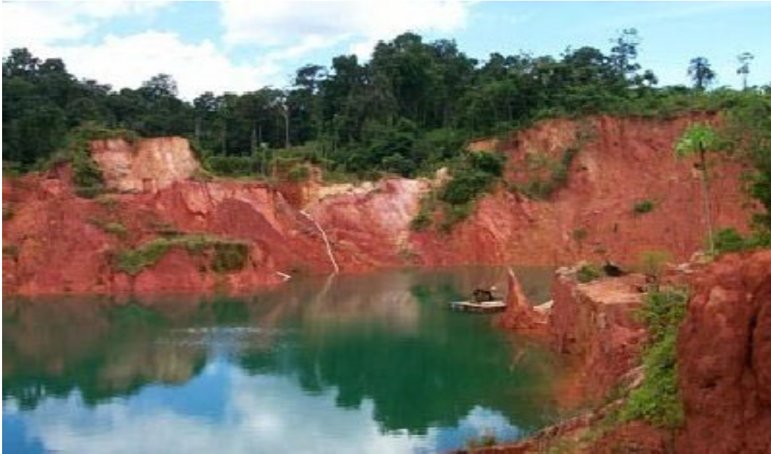
Figure 2: An example of ‘good’ mining practice. Water discharged from the Tailings Pond indicate very low level of sediments. (Pictures with compliments of GGMC)
